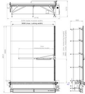
Table of basic dimensions of US-1 cutting tables depending on the selected table module length (for max. cutting width 3000mm)
