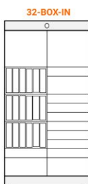
32-BOX-IN additional module V - 18 (61x655x260 mm) S - 9 (440x655x93 mm) M - 3 (440x655x201 mm) L - 2 (440x655x417 mm)
